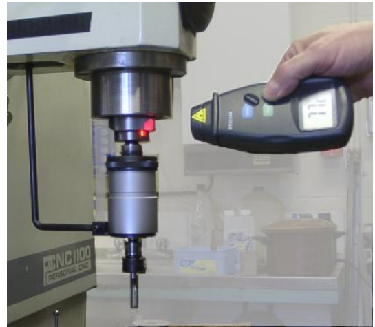
Figure 8.27 – Measuring spindle speed
