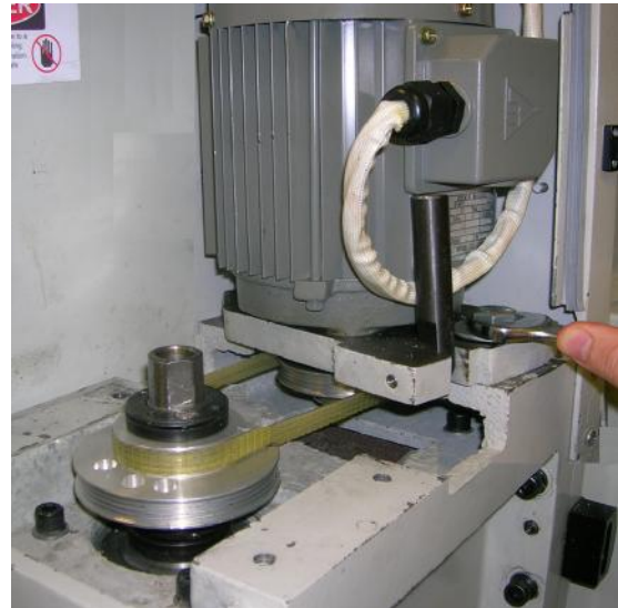
Figure 5.8 – Changing spindle speed range
