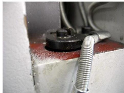
Figure 9.1a – Upper Z gib screw
