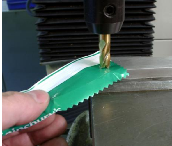
Figure 6.11 – "Roll-your-own" gauge in use
