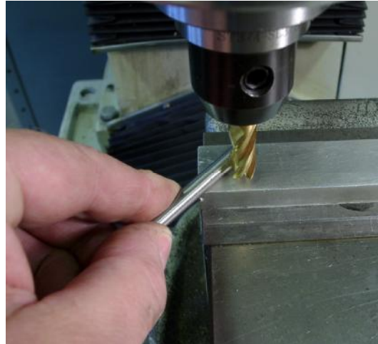
Figure 6.12 – Tool much too low for gauge
