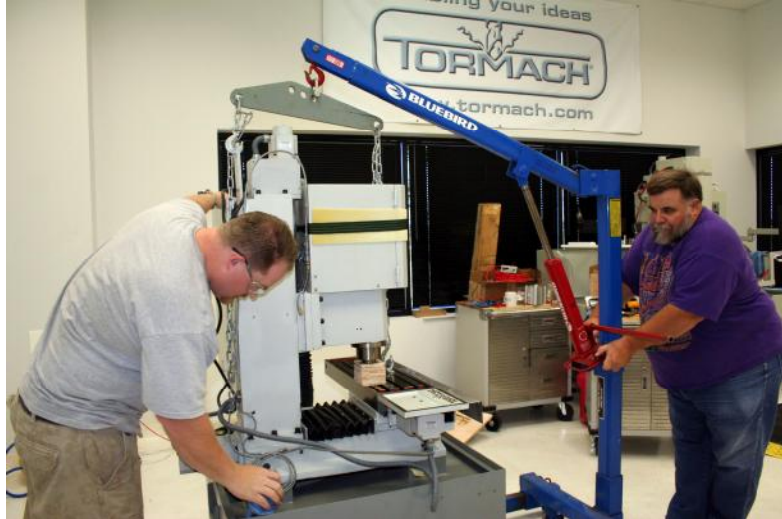
Figure 2.5 – Hoist bar for slinging the mill
